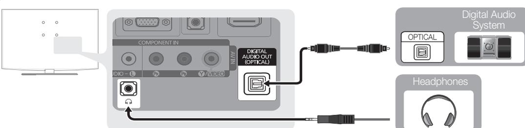
The diagram shows a TV's rear panel with various audio ports. A cable connects the TV's **DIGITAL AUDIO OUT (OPTICAL)** port to a **Digital Audio System** (which has an **OPTICAL** input). Another cable connects the TV's **AUDIO** (analog) port to a pair of **Headphones**.
